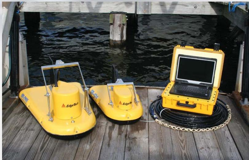
The 3100 is EdgeTech's portable version of their highly successful sub-bottom profiler product line. The system utilizes EdgeTech's Full Spectrum CHIRP technology which provides higher resolution imagery of the sub-bottom structure and greater penetration.
